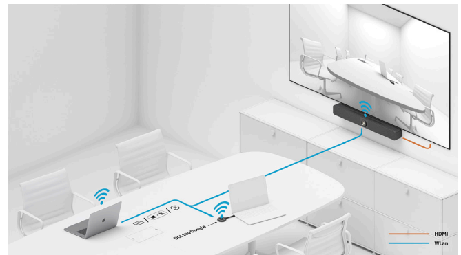
4. Using the VB300 as a pure presentation and collaboration solution without a conference room PC.
