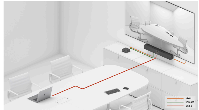
2. Using the VB300 in combination with a conference room PC for video conferences without own hardware or with own hardware BYOM e.g. own laptop.
