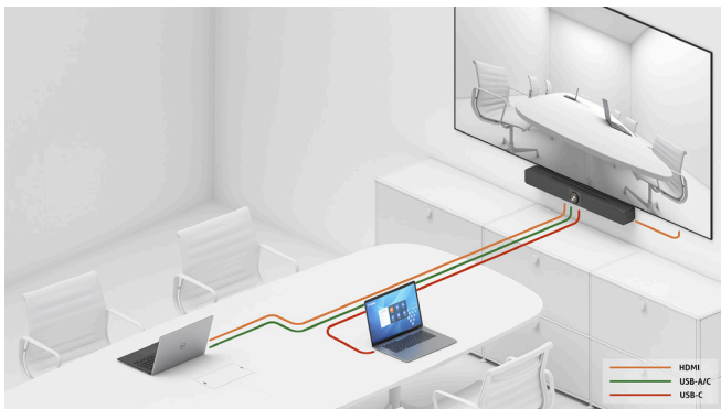
3. Using the VB300 via USB-C (BYOM) without a conference room PC
