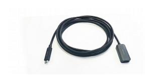
CA-USB31/CAE is an active extender cable designed to extend USB 3.1 GEN 2 (USB 3.2) signals. Typically, USB 3.1 GEN 2 cables have a maximum length of about 1 meter (3 feet), CA-USB31/CAE enables cable lengths of up to 4.7m (15ft).
