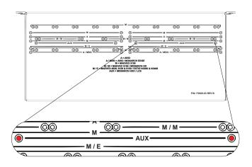
NOTE: Secure the angled brackets to the Monarch *before* attaching to the mounting shelf. Use the lower screw holes for Monarch HDX and Monarch LCS.
