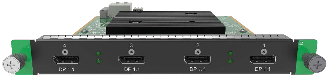
Figure 5-16 DP 1.1 quad input card
