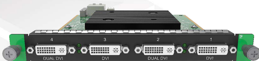
Figure 5-11 SL-DVI quad input card
