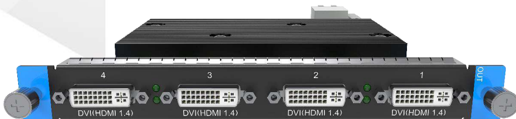
Figure 5-20 DVI (HDMI 1.4) quad output card
