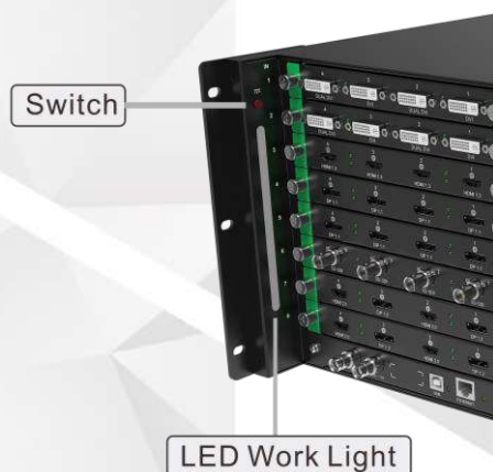
Figure 5-9 LED work light on one side of rear panel
