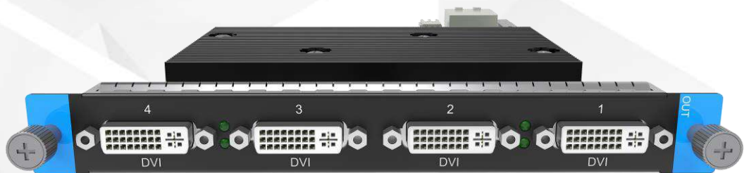
Figure 5-18 SL-DVI quad output card
