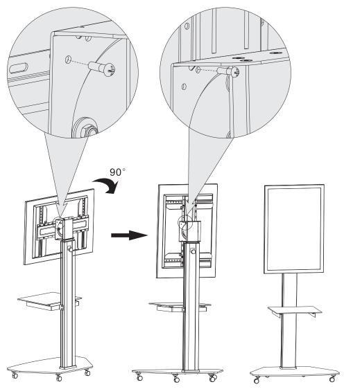
Remove the screw on the top plate to rotate the TV (withe attached brackets and top plate  $90^{\circ}$ , Secure with just removed screw in another position.
