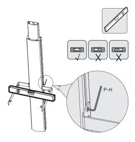
Make sure both support arms are on the same level and tighten all screws to secure them.
