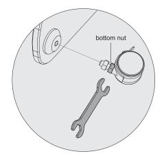
Install the casters into the base holes and tighten bottom nuts of casters at the desired height.
