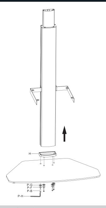
Attach the column and the foot pad to the base using the correct screws and washers. Tighten all screws with Allen key.
