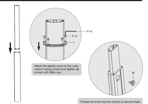
Insert the inner column into the outer column at the desired position.
