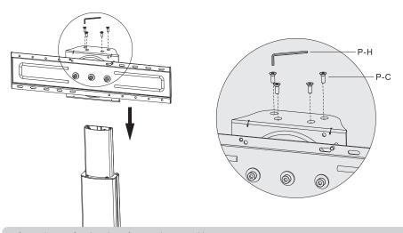
Insert the top plate into the column and secure with screws.
