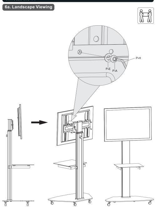
Attach the TV to top plate with the appropriate combination of screws and washers.
