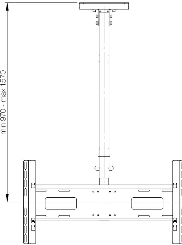
Minimum and maximum lengths standard pipes + extension pipes 1:
