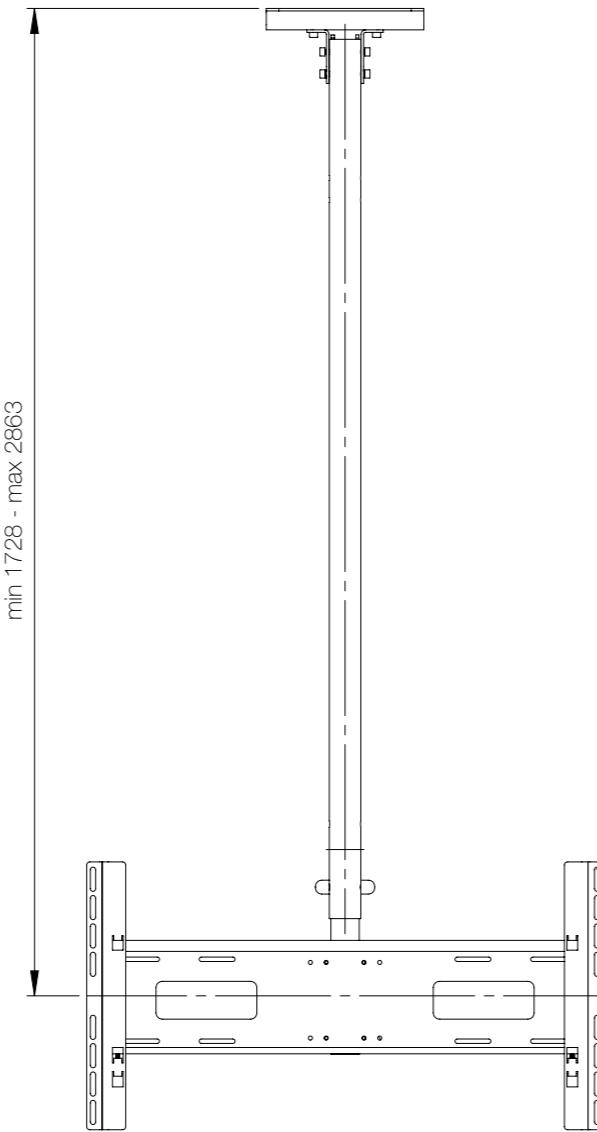
Minimum and maximum lengths standard pipes + extension pipes 2
