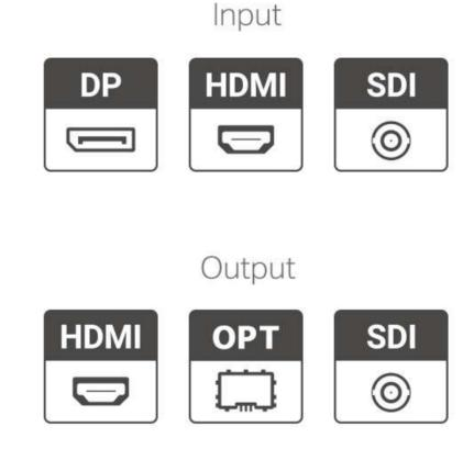
HDR Master supports flexible interface choices, includes: one swappable input card: DP1.2×1, HDMI2.0×1, 12G-SDI×4 and two swappable output cards: one contains HDMI2.0×1, 10G optical fiber×4 and one contains HDMI2.0×1, 12G-SDI×4.
