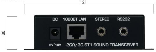
All measurements in millimeters (mm)
