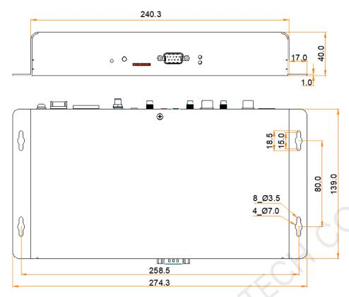
Tolerance: ±0.3 Unit: mm
