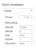
RS232 settings can be done for multiple devices simultaneously using the Multi-device settings option. For more information, see "6.9 - Modify settings", page 56.
