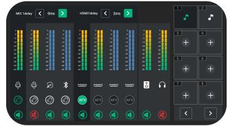
2. mini-mx supports audio output mix of multiple channels. You can turn on/off analog audio output and the volume can be adjusted by Channel Fader. 10 audio columns indicate MIC1\MIC2\LINEIN\Bluetooth\HDMI1\HDMI 2\HDMI3\HDMI4\PGM\Monitor respectively. If the sound and the video are not synchronous, increase or reduce the Delay value.
