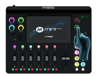
Push the MENU button and the 5.5-inch LCD screen will quickly enter the main menu interface. The right part of the screen displays the main menu interface, as shown in the right figure.
