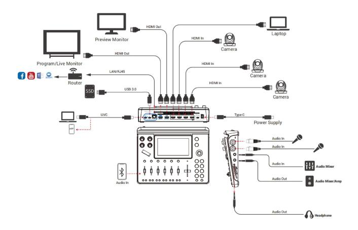
mini-mx System Connection Diagram
