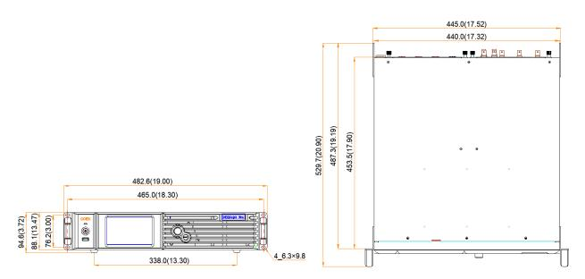
Tolerance: ±0.5 Unit: mm
