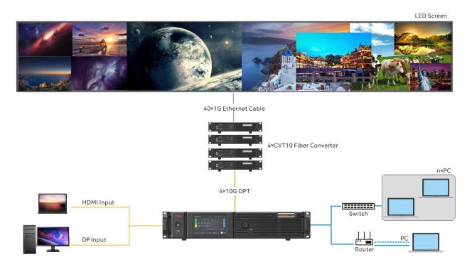
This diagram is an example of two input cards and one MX\_4x10G\_Fiber output card installed on an MX2000 Pro. The actual application may vary.
