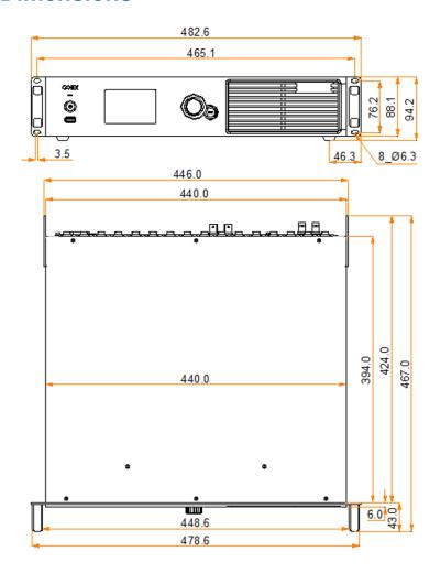
Tolerance: ±0.3 Unit: mm
