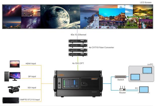
This diagram is an example of four input cards and one MX\_4x10G\_Fiber output card installed on a MX6000 Pro. The actual application may vary.
