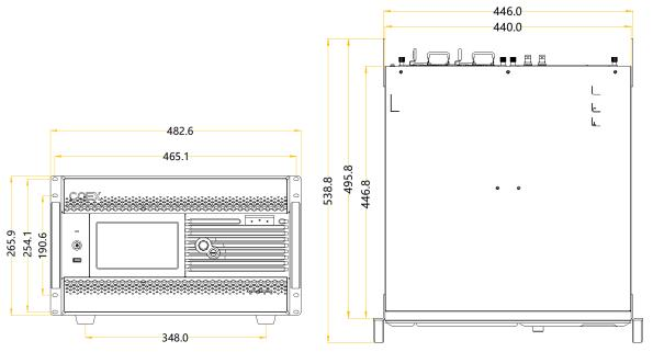
Tolerance: ±0.3 Unit: mm
