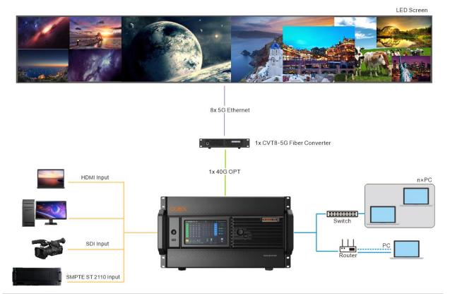
This diagram is an example of four input cards and one CX\_1x40G\_Fiber output card installed on a MX6000 Pro. The actual application may vary.
