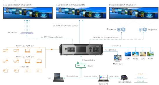
Figure 4-2 PGM only mode (P20+U5+PixelFlow)
