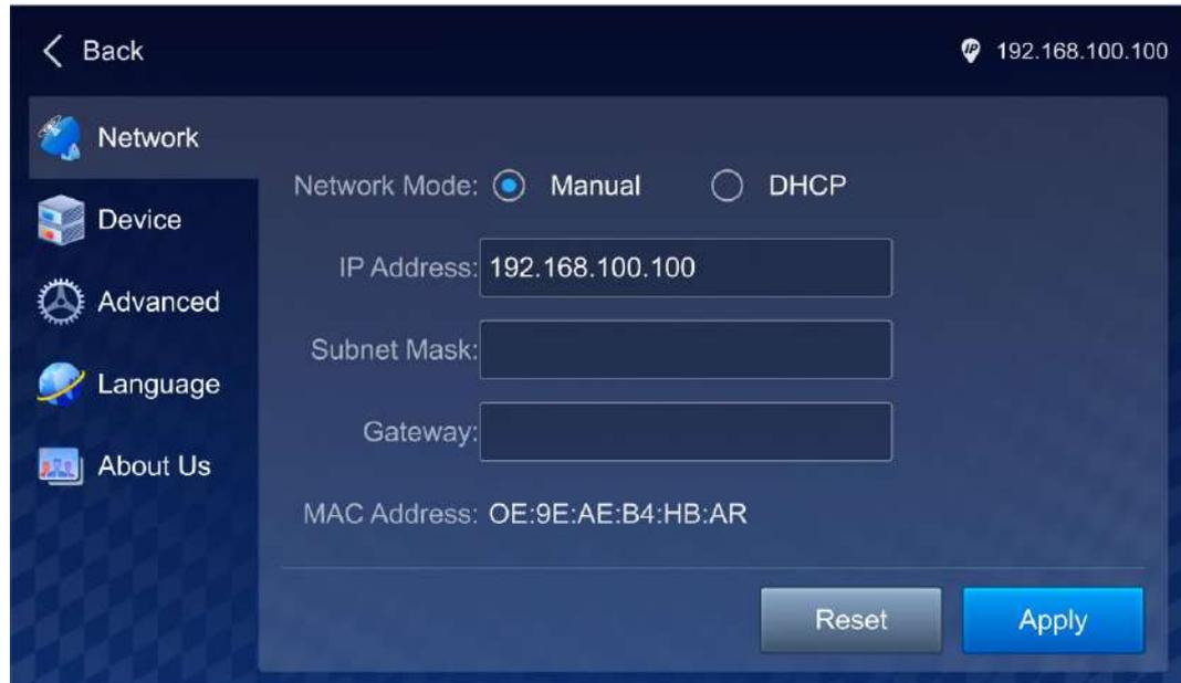
The device supports both automatic (DHCP) and manual IP configuration. When the device is connected via router or switch, DHCP is recommended. The router or switch will automatically assign IP address to the device. When the network mode is set to **Manual**, you need to set **IP Address**, **Subnet Mask** and **Gateway**.
