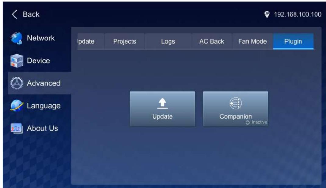
The Q8 supports plugin update via USB drive. To do that, first save the update file in the root directory of the USB drive, and then insert the USB drive into the USB port on the control card of the Q8.
