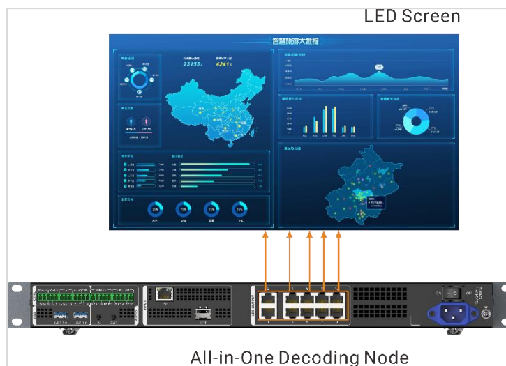
Figure 2-7 LED screen connections
