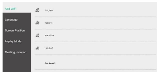
Click "Add WIFI" and select the network to be added from the WIFI list. After joining the network, the screen of RX will display the name of the LAN and the IP address
