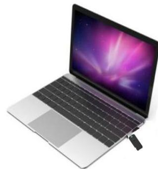
**Note:**if projection is unsuccessful,unplug the TX, and supply power to TX's HDMI port via microUSB-USB cable and power adapter.then connect TX's HDMI port to the PC's HDMI port again.touch the projection key to project.
