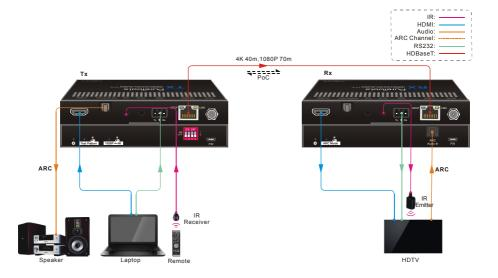
**Note:** The STP cable is recommended to be used to ensure optimal machine performance in ARC mode.
