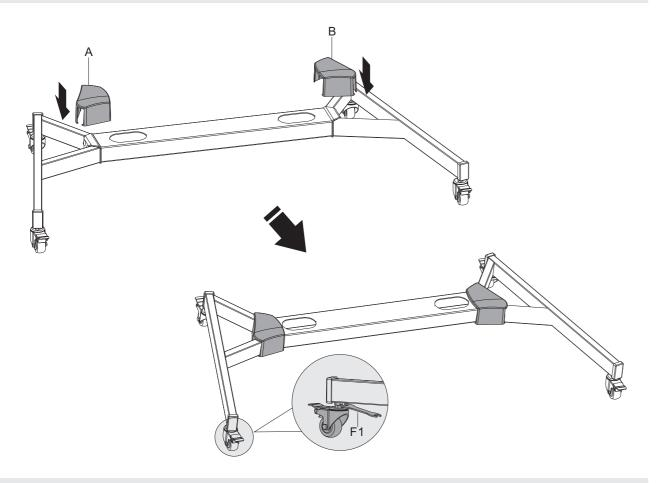
**NOTE:** Lock the brakes on the casters to avoid any unexpected movements during installation. Each caster can be adjusted independently for fine tuning. Slightly turn the nut to lower or raise the base.
