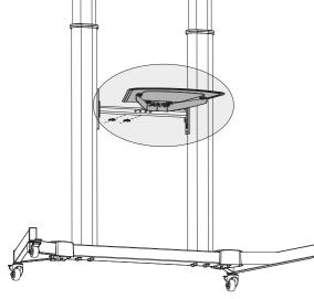
Attach the DVD shelf to the support bar with the appropriate screws and butterfly nuts. Tighten all screws and butterfly nuts to secure.
