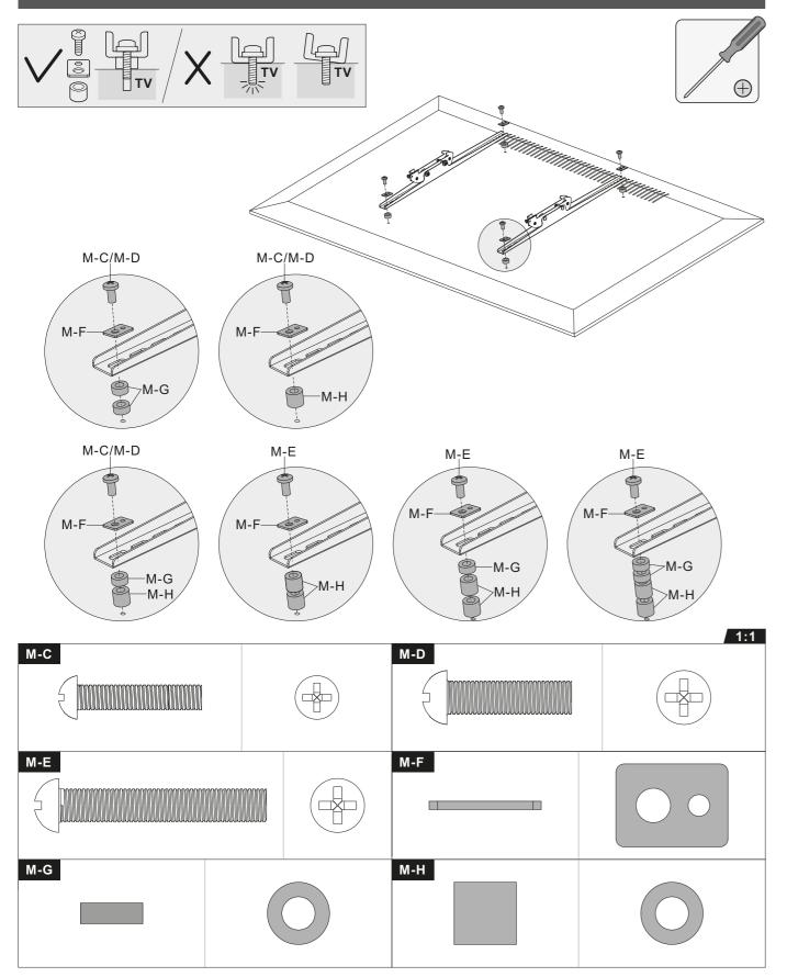
Note: Choose the appropriate screws, washers and spacers (if necessary) according to the type of screen. Position the adapter brackets as close as possible to the center of the display. · Screw the adapter brackets onto the display.
