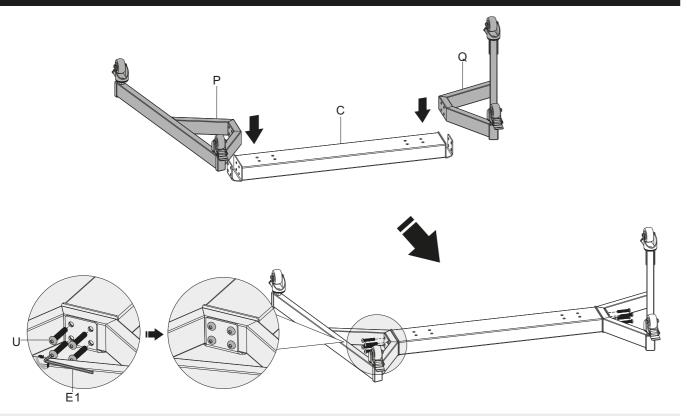
Attach the right base to the middle base and secure with screws(U). Repeat this step for the left base.
