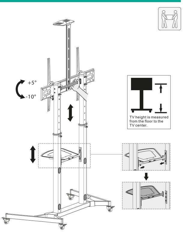
It is recommended to adjust the columns to the desired height before installing the display.
