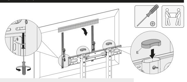
· Hook the display onto the universal plate. • Tighten the bottom screws to secure them. IMPORTANT: Make sure the display is mounted correctly and the screws are tightened safely before releasing the display.
