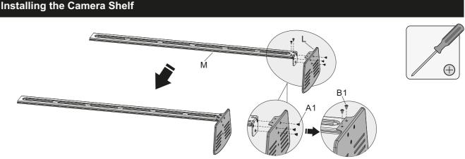
Attach the camera shelf to the connecting plate with the appropriate screws. Tighten all screws using a proper Phillips screwdriver.
