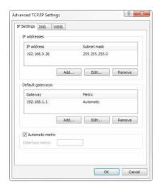
Note: The IP address to be added cannot be same with that of other computers or devices. The existence of this IP address needs to be verified before adding
