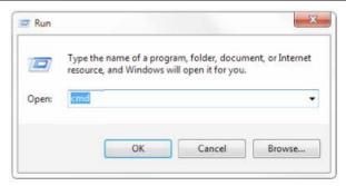
4) Click "OK" and open the DOS command window, input ping 192.168.5.26 and press Enter key, it will show message as below:which means network segment adding is succeed.
