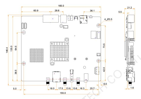
Tolerance: ±0.3 Unit: mm
