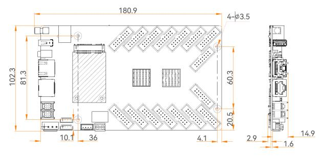
Tolerance: ±0.3 Unit: mm
