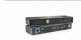
TP-590T is a high-performance, long-reach HDBaseT 2.0 transmitter for 4K60Hz (4:2:0) HDMI, USB, RS-232, and IR signals over twisted pair. TP-590T converts all input signals into the transmitted HDBaseT 2.0 signal. It extends video signals to up 40m (130ft) over CAT copper cables at up to 4K@60Hz (4:2:0) 24bpp video resolution and provides even further reach for lower HD video resolutions
