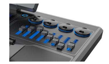
Four encoders and eight faders make the event operations amazingly convenient. Also, the encoders and faders can be bound with external MIDI functions for volume adjustment and more.
