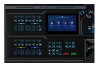
User-programmable LCD function buttons satisfy all your operation requirements in the field. Function names, pages and more can be clearly shown on the buttons, and the button skins and styles can be customized as you wish.
