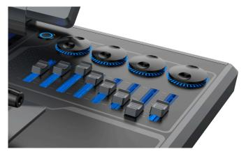
Four encoders and eight faders make the event operations amazingly convenient. Also, the encoders and faders can be bound with external MIDI functions for volume adjustment and more.
