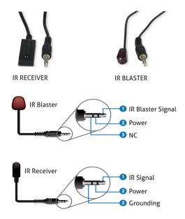
**Note:** The frequency of the blaster and receiver component and the pin out of the IR cables is 20-60KHz.
