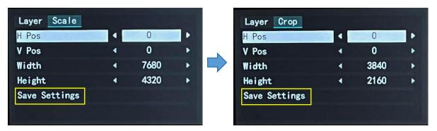
Type horizontal position, Vertical position, Width and Height as needed. Then click "Save Settings" > "Confirm" to save above parameters.
