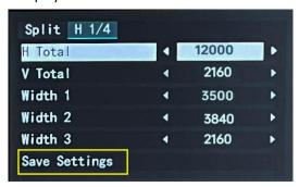
Set H Total, V Total, Width 1, Width 2 and Width 3 of screen according to actual need.
