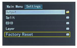
Performing a factory reset will delete all user data and personalized settings on the device and return it to its initial state.
