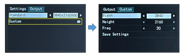
D8 supports to customize output resolution. If you set the resolution to 3840x2160@50, type in Width, Height and Frequency one by one and click "Enter" to save. Then check the set resolution in <Device> interface.
