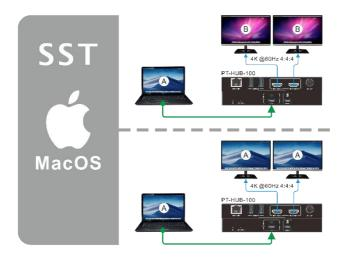
In SST\*\* mode, the HDMI outputs support up to 4K 60Hz (4:4:4) resolution.
