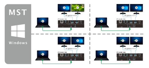
In MST\* mode, the HDMI outputs support up to 4K@60 4:4:4 resolution.
