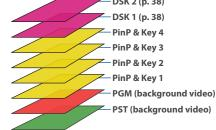
• Long-pressing the [PVW] or [PGM] button for each layer shows only the layer that is targeted for the operation while the button is pressed
