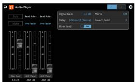
**3.** Touch the screen to configure the send amount for each bus. On page 2, you can configure the effects as with the other audio channels.
