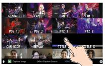
\* To capture the output video, set the Monitor setting to "Program" (by pressing the [Program] button), or switch to multi-view (by pressing the [Multi-View] button) to select an output video, or use Select Capture Source to select the output video.
