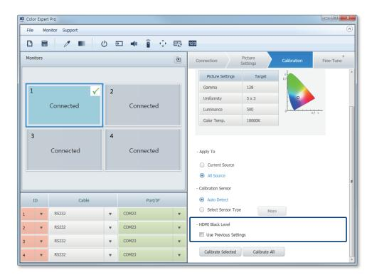
3 After configuring the settings, start calibration. For further details, refer to the following: ► Calibrating devices
