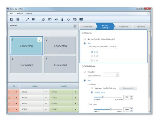
Uniformity Size (Horizontal X Vertical) Specify the number of columns and rows to split the screen you want to calibrate the uniformity for.
